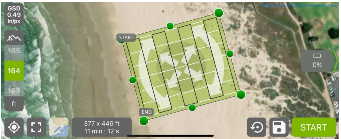
Figure 2. An example of the double grid flight path that I pre-programmed the drone to fly.
